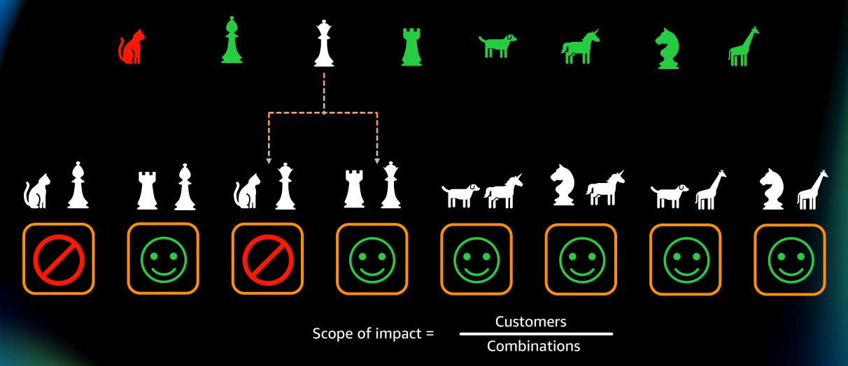
\*retry logic in the client to try every endpoint in a Shuffle Shard, until one succeeds
