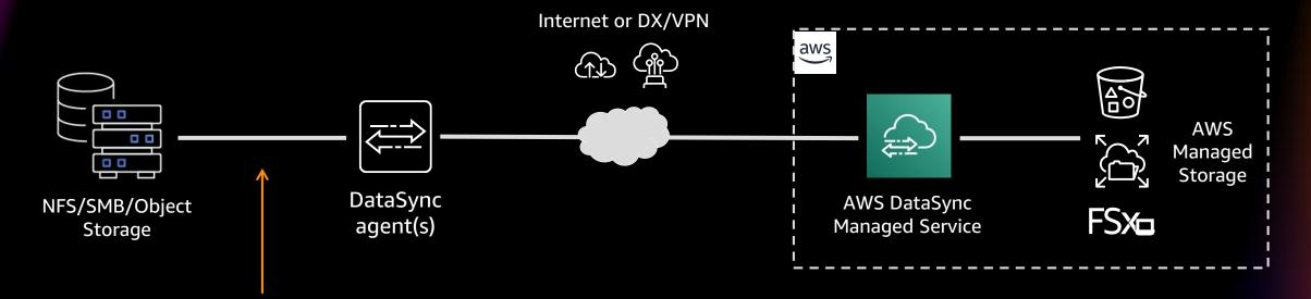
This needs to be fast and low latency. Install the agents as close to the customermanaged storage as possible
