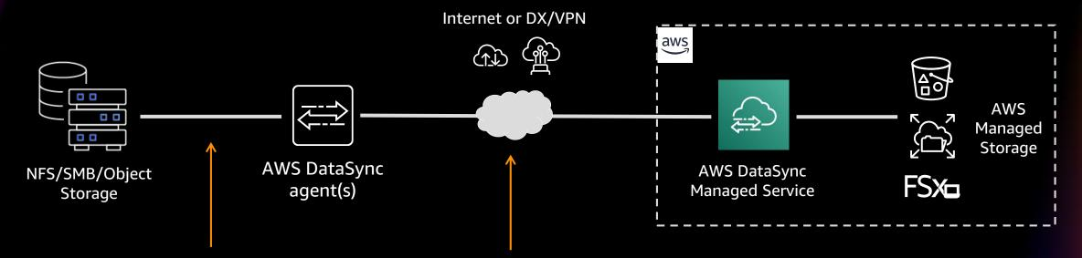
This needs to be fast and low latency. Install the agents as close to the customermanaged storage as possible
